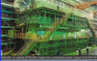
Wärtsilä's 14-cylinder RT-flex96C engine has a maximum power output of 96,000 kW
